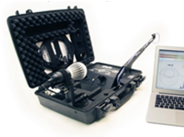
Figure 50. Photograph of the LightSpion test suitcase testing an LED lamp
